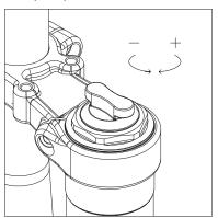
Main air chamber Fill in the air according to suggested pressure meter.
